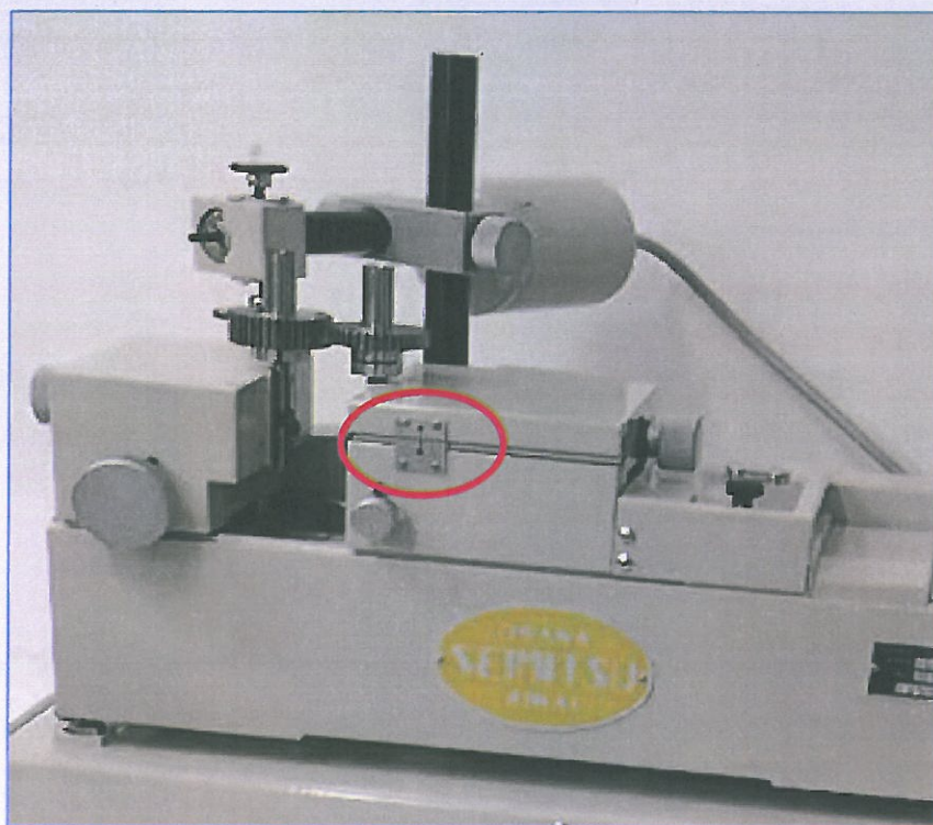
图 12 安装了标准齿和产品后，旋转滑动基体的进给旋钮，直到产品与标准齿轮紧密咬合，且定位器显示为一条直线。 Picture 12 After mounting master gear and work gear, turn 'Feeding Knob for sliding base' until the the tooth of the product is meshing tightly with the master gear and the position index is approximately in a line.
